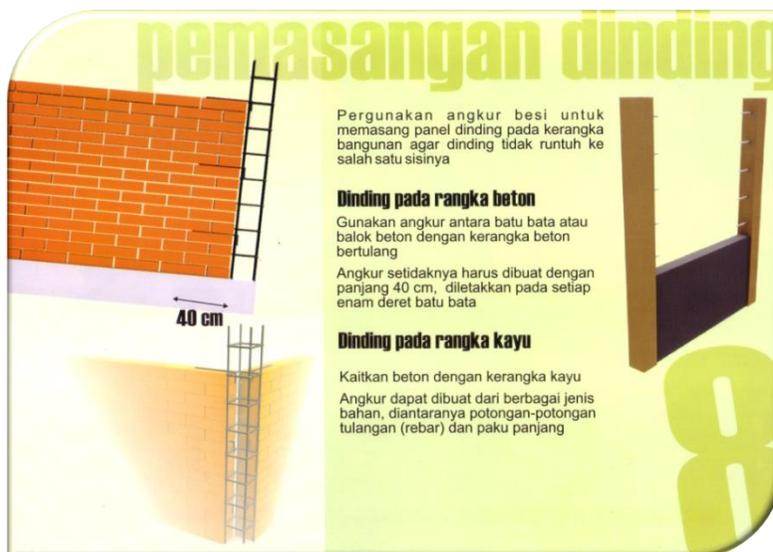
Gambar 42: Pemasangan Dinding
